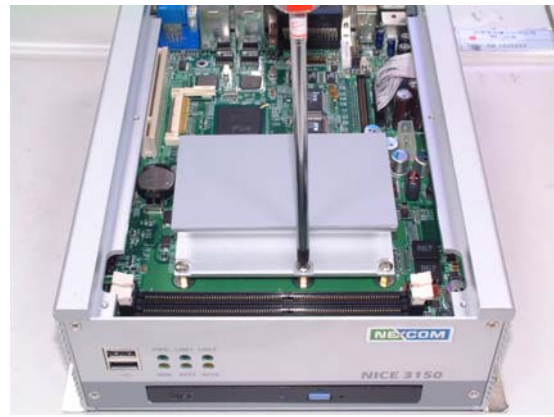
Step 2.5: Lock the heat sink with screw
