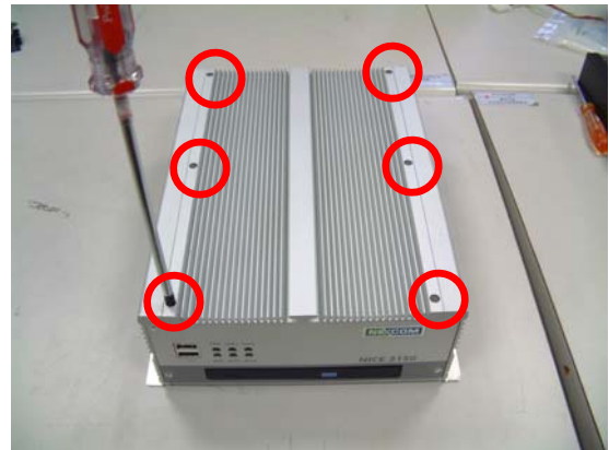
Step 4: Secure the top cover with screws
